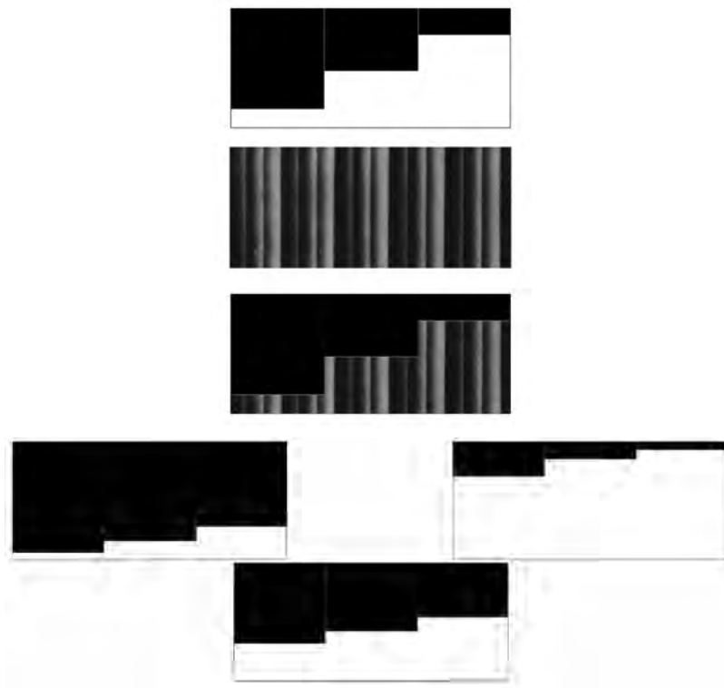
fig 7.44 A bell-like mask to create an amplitude envelope (left) and the way to crossfade successive frames (right). Diagram by A. Smirnov.
